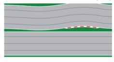
There is initially a slight pivot inwardly (2 cm) and then a somewhat clearer pivot swing outwards (4 cm). The smallest radius is located at the exit of the curve, and is 1.35 m. The curves are performed as splines. At the entrance of the curve you are greeted with a very large radius of 5.85 m, towards the end, the radii then close. Depending on the voltage can be very fast, but do not go full throttle.
