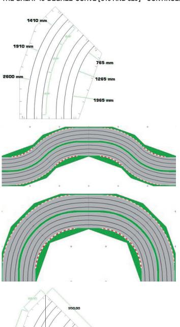
The distance between the marking crosses is each 85 cm. An S-curve of two 45-degree modules is 2.55 m ( $3 \times 85$  cm) long and 1.70 m wide ( $2 \times 85$  cm). The modules are ideally installed in the 85-cm increments. Overall this double-S curve is 5.10 m ( $6 \times 85$  cm) long.
